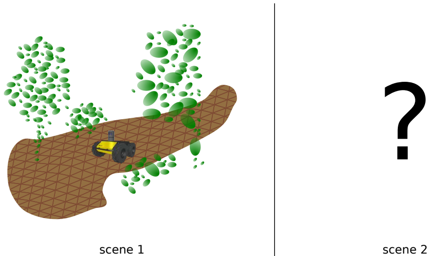
FIGURE 4.4: The hybrid geometric simulator models terrain with a combination of surface meshes and Gaussian distributions. These are fit to data. However, it is geo-specific, and new scenes cannot be simulated.
